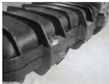
The side of the closure after sealing
